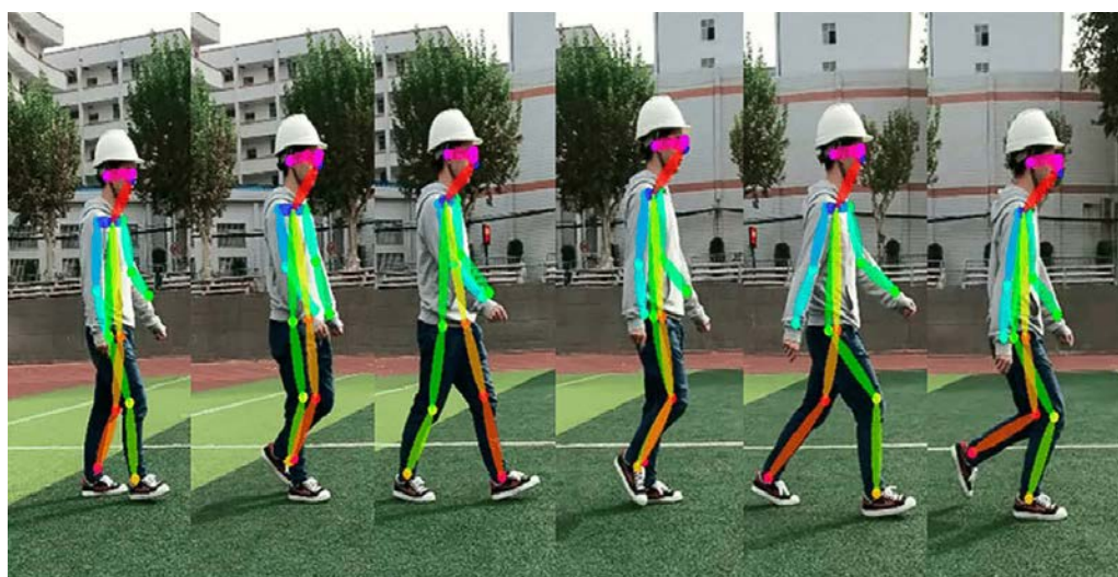
Figure 4. Fall Detection Based on Key Points of Human-Skeleton Using OpenPose (Chen [et al.], 2020).
